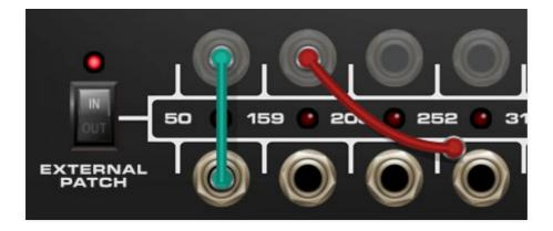
To patch a cable, simply click and hold on a jack then drag to another jack and release the mouse button. Cables can be routed from an input to an output, or from an output to an input. When a cable is being dragged, all potential destinations will appear normal, and non-destinations will gray out this prevents inputs from being routed to other inputs and outputs from being routed to other outputs.
