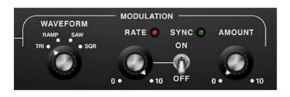
The Modulation section allows low-frequency oscillator (LFO) modulation of Shift Amount.
