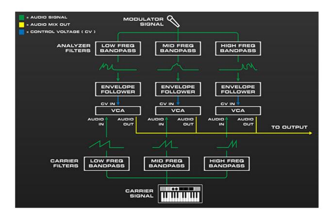
As mentioned, a vocoder imparts the frequency spectrum of one sound onto another. In the diagram above, a microphone's frequency spectrum (i.e., speech), is imparted onto the sound of a synthesizer playing a basic sawtooth-wave patch. Let's break down what's happening:
