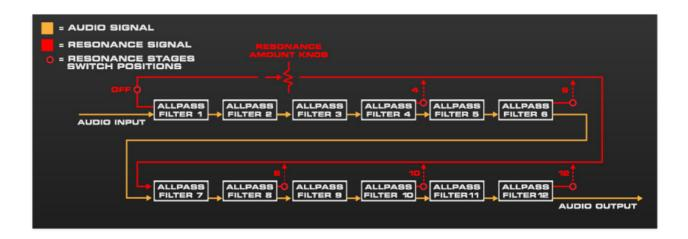
**Resonant Stages selector / Resonance knob**- The phased signal can be fed back into the allpass filter chain to intensify the phasing effect. The *Resonant Stages* selector chooses where the feedback signal is tapped; the Resonance knob adjusts the amount of signal fed back through the chain.
