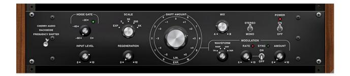
The Cherry Audio Rackmode Frequency Shifter is a super-accurate recreation of the vintage Bode Frequency Shifter. A frequency shifter is an audio modifier that "shifts" the entire frequency spectrum of the signal by a given amount. The Rackmode Frequency Shifter can shift the spectrum up or down by up to 5000 Hz, and the "downshifted" and "upshifted" signals are simultaneously available. The shift amount can be modulated via the onboard low-frequency oscillator.
